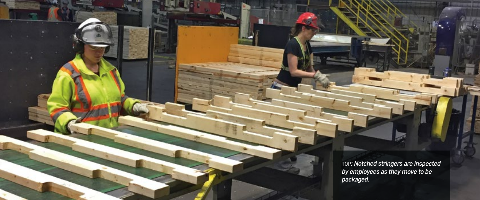
CENTRE: Pallet deck boards being graded before they are packaged for shipping to customers.
