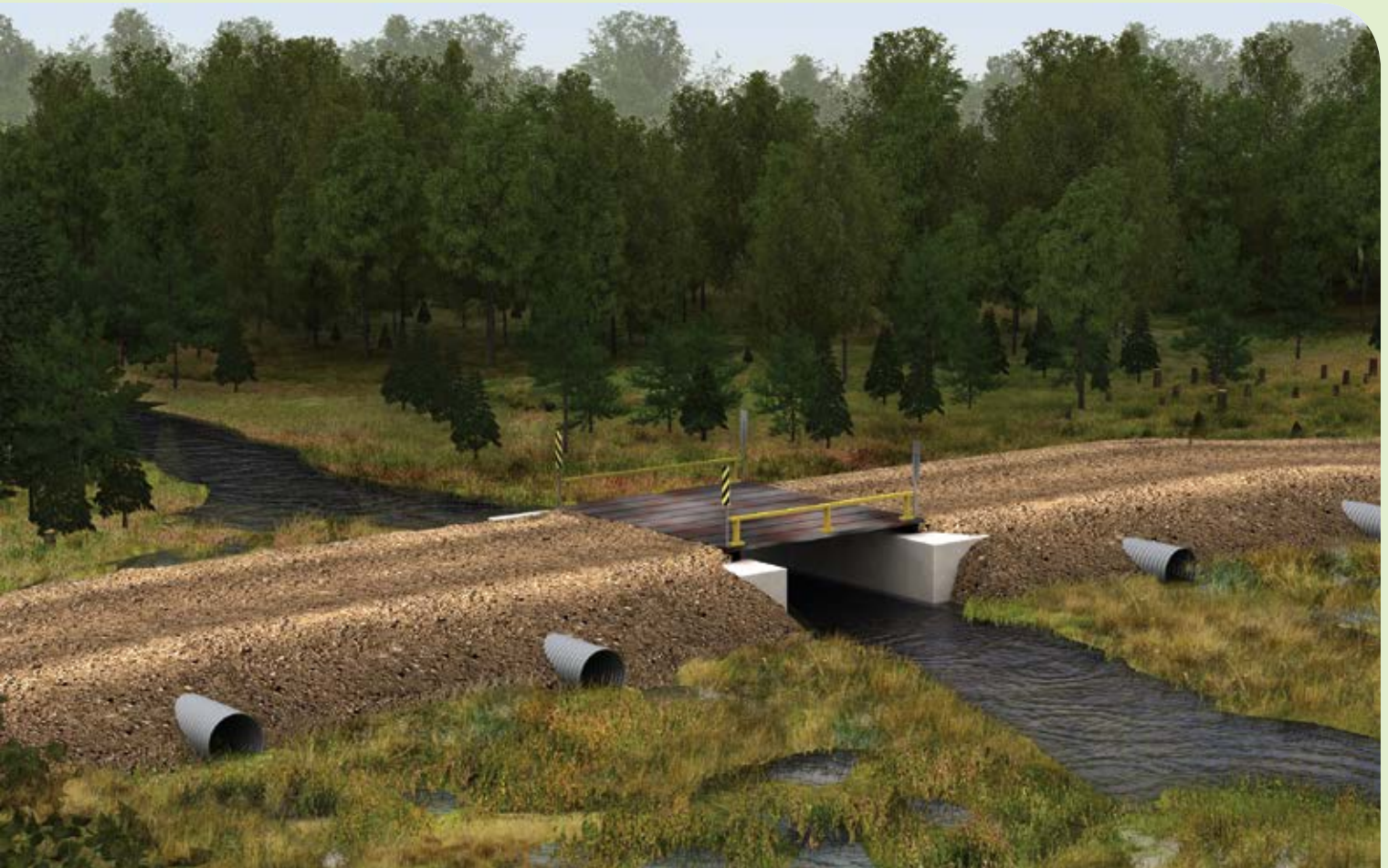
ABOVE: Culverts may be installed in the approaches to defined water crossings to enable hydrologic connectivity of the wetland.
