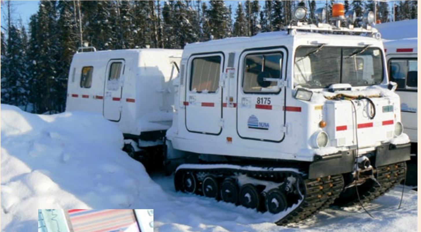
Above: Häggglunds amphibious vehicles are used in early stages of ice bridge construction.
