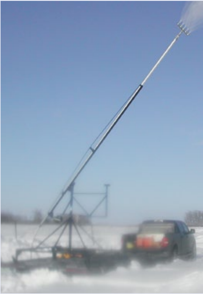
Figure 2. Airless system used for making snow.
